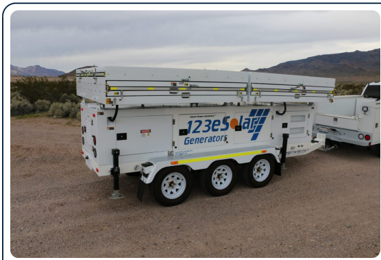
123-STG-72D62 Engine 10.8 h a day, the sun and the battery the rest · 12.2 gal a day
