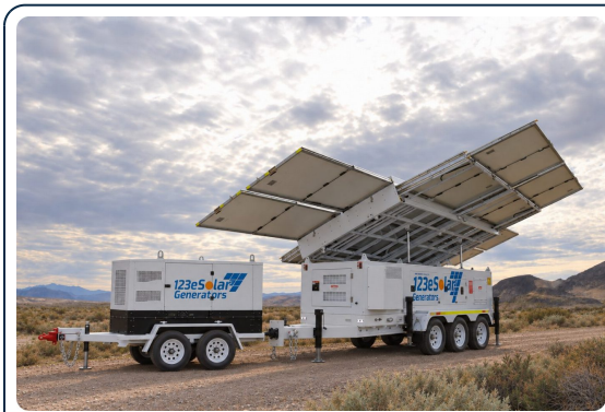
123-SG-7S82-40 Engine 6.2 h a day, the sun and the battery the rest · 8.4 gal a day
