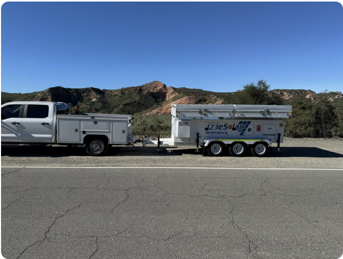
The 123-SG-7D63 under tow on the highway shoulder: 16 panels folded flat over the enclosure, three axles beneath it and the jacks up for the road.
