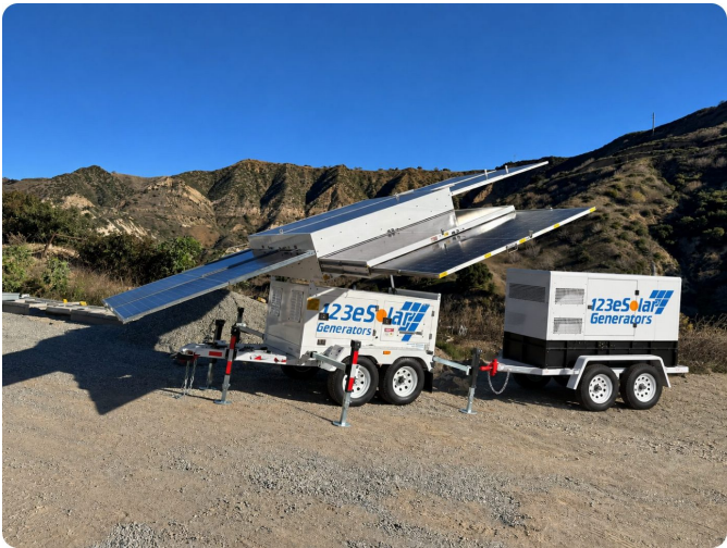
Two units, one system: ten panels open beside the standalone 40 kW diesel.
